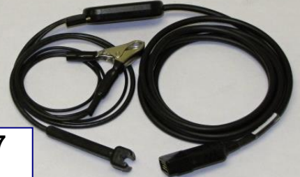
HV probe C1 AT111 4017 with reference cable
